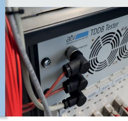
The TDDB / HTRB HV Tester is used for long-term measurements with high voltage dc bias. During this long-term measurement, an adjustable bias voltage is applied to the DUTs (Device under Test). In an adjustable measuring interval, all measuring channels are measured sequentially and stored as a data set.
