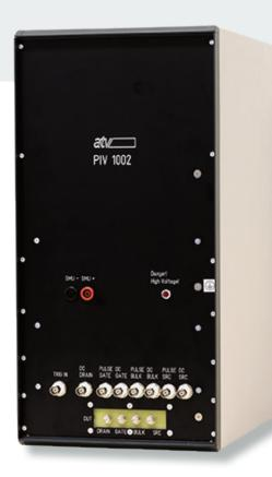
PIV 1002 is a laboratory system for the characterization of high-voltage MOSFET. The system is designed to be carried out on MOSFET pulsed measurements at high voltages and currents. As a result, characteristic curves are recorded without overloading the device thermally.
